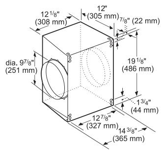
measurements in inches and mm
