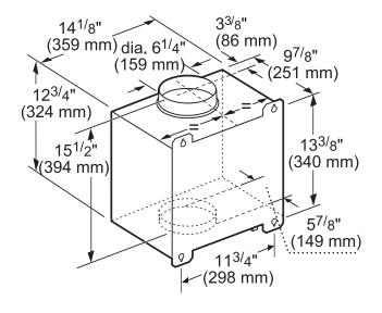
measurements in inches and mm
