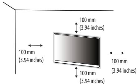
To install the monitor to a wall, attach a wall mounting bracket (optional) to the back of the monitor.
