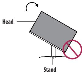
3 Rotate the monitor clockwise as shown in the figure.
