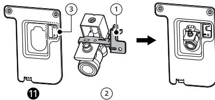
**3** Fasten the valve cover **11** to the bracket with 1 Phillips screw **7**.
