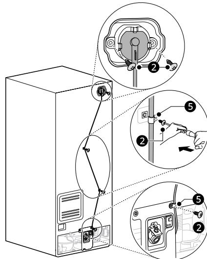
**4** Assemble the valve cover on the refrigerator.
