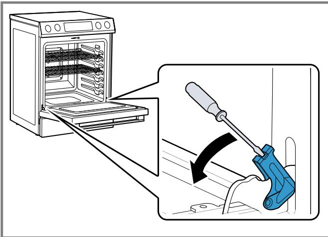
3. Slowly close the door to a 10° angle from the fully closed position, then pull the door away from the oven.
