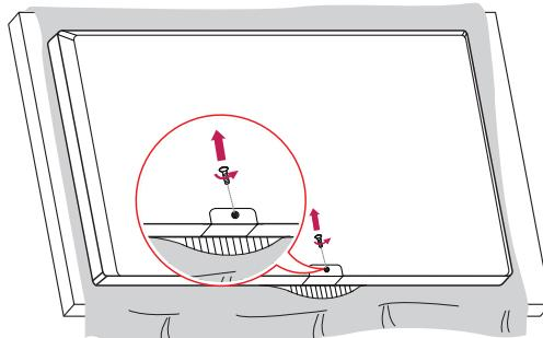
2 After removing the screw, remove the LG Logo Bracket. Align with the hole on the left side to attach the LG Logo Bracket with a screw.
