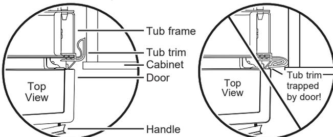
Tub trim may be trimmed if necessary to ensure proper door operation
