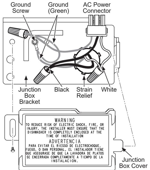
**NOTE:** All ground screws, brackets and wires must remain intact.
