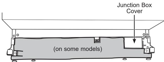
Insulation shown correctly placed along the bottom edge of the control box, the dishwasher bottom and flush with the front face.
