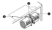
6 Attach the blower plate 4 to the microwave oven so the blower unit exhaust ports 3 and blower plate opening are aligned. Attach one or two blower unit mounting screw(s) 6 and then one or several blower plate mounting screw(s) 1. Attach the cover plate 7 on the blower plate with a screw 3.
