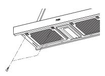
To remove, slide the grease filter forward slightly and pull it downward.
