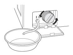
**5** Clean the pump filter and opening.
