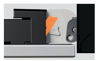
3. Locate the hinge locks on either side of the door. Push the locks upwards to release. Holding the door on both sides, partially close the door and carefully pull the door away from the hinges.
