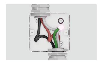
**5.** Connect the factory-taped green and white oven wires to the neutral (white) wire in the junction box.
