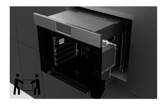
1. Ensure water tank is locked in place. Lift product into cavity taking care not to lift from the control panel.
