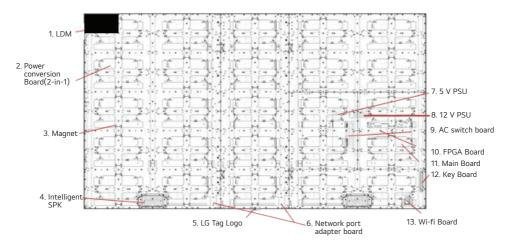
Figure 2.1 Major components placement for LAPA136-GF
