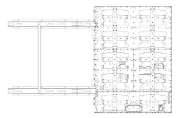
2 Place the half screen component on the Wall Mount structure in order.
