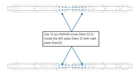
Step2. Install the left and right plate Components with vertical connection plate.
